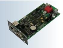
The NetMan Plus network agent allows UPS management across a LAN using any of the main network communication protocols - TCP/IP, HTTP and network interface (SNMP). NetMan Plus enabled UPS integrate easily into medium and large sized networks and provide reliable communications between the UPS and management systems employed.
