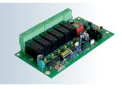
The I/O expansion card, for the Master Plus range, is equipped with:
