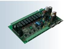
Multi I/O has configurable input and output signal contacts to allow UPS integration with control systems. It can be used to connect two devices to a single UPS serial communication port. It can also communicate using the MODBUS/JBUS protocol on RS485 lines.
