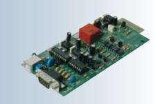
MultiCOM 362 provides a UPS with an additional RS232 serial interface or USB port. The USB port allows the UPS to communicate with Apple Macintosh computers as well as Windows and Linux operating systems.
